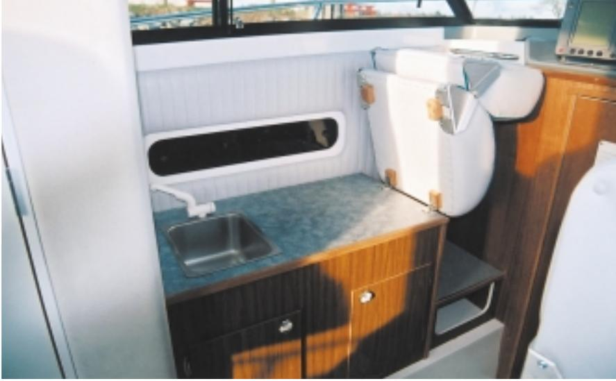
Above: The mate's seat tilts forward to provide additional counter space.
